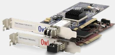
Owl V7 Data Diode Card Kits are comprised of two purpose-built network interface cards (one send, one receive) connected via a fiber optic cable. Each individual card is installed on a separate host server in a PCIe slot. Owl V7 cards facilitate high bandwidth, low latency one-way transfer at up to 10 Gbps.
